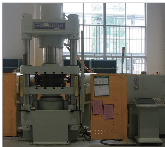
Fig.4 Cold expansion push-bending forming equipment
