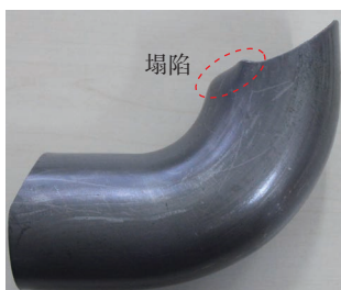
图 12 高温合金冷胀推弯常见的塌陷缺陷 Fig.12 Common collapse defects in cold expansion push-bending forming of superalloys
